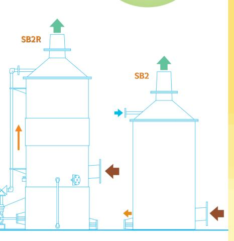
ng static storage and pumped discharge, the SB2 is NOT ring deliveries above 7 psi from air pressure tanker discharge
