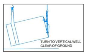
From the "main" crane, attach lifting chains to the lifting points at the top of the tank in the same manner as above, ensuring that the lower lugs take the initial weight of the lift. Use a "tailing" crane to lift the lower end of the tank, using a minimum 150mm wide fabric sling. Pass the sling round the lower girth of the tank and make a "noose" by passing one looped end through the other. To prevent the sling slipping up the wall of the tank as it is turned to the vertical, you can tie a
